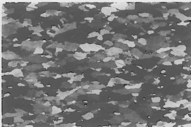
Fig. 4 - Micrograph of ultrathin section of dynamic recrystallized Carrara marble (microstructure type B1, sample B, Arni). The grain shape define the main foliation in the outcrop (a differentiated crenulation cleavage in pelitic layers). XZ plane, length of micrograph 1,6 mm cross polarized light.
