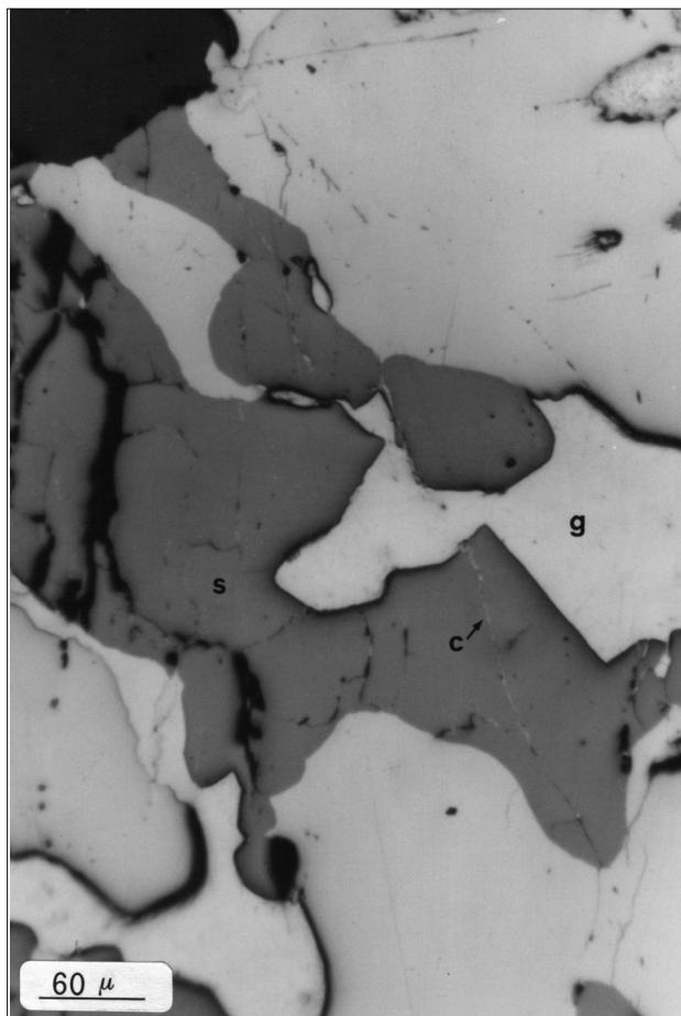
Fig. 3 - Galena (g) and sphalerite (s) with inclusions of chalcopyrite (c). Reflected light observation.
