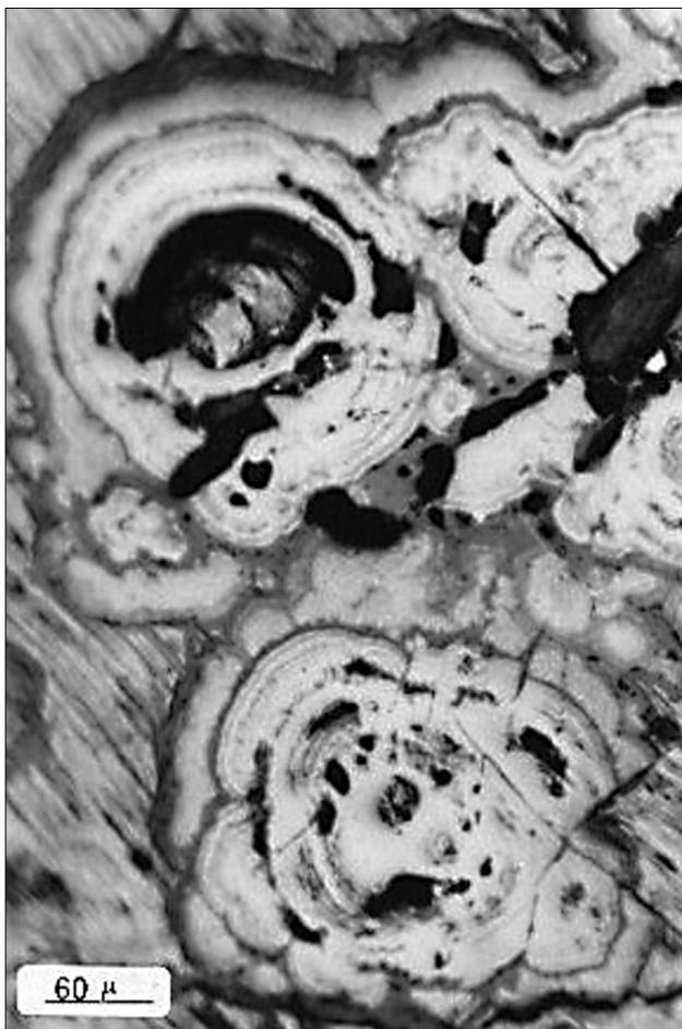
Fig. 2 - Typical pyrrhotite alteration known as "Bird's eye". Reflected light observation.
