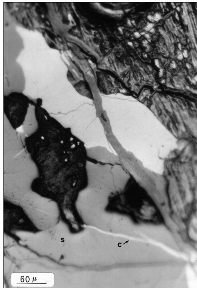
Fig. 4 - Chalcopyrite (c) as filling of the fractures inside sphalerite (s). Reflected light observation.
