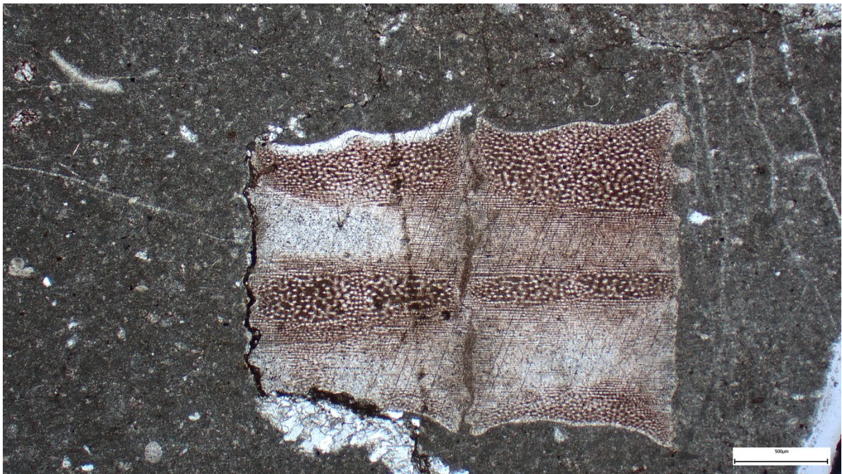
d) MOS 4B - Rosso Ammonitico Fm. Abraded echinoderm plate. Plane polarized light, scale bar: 500 μm.
