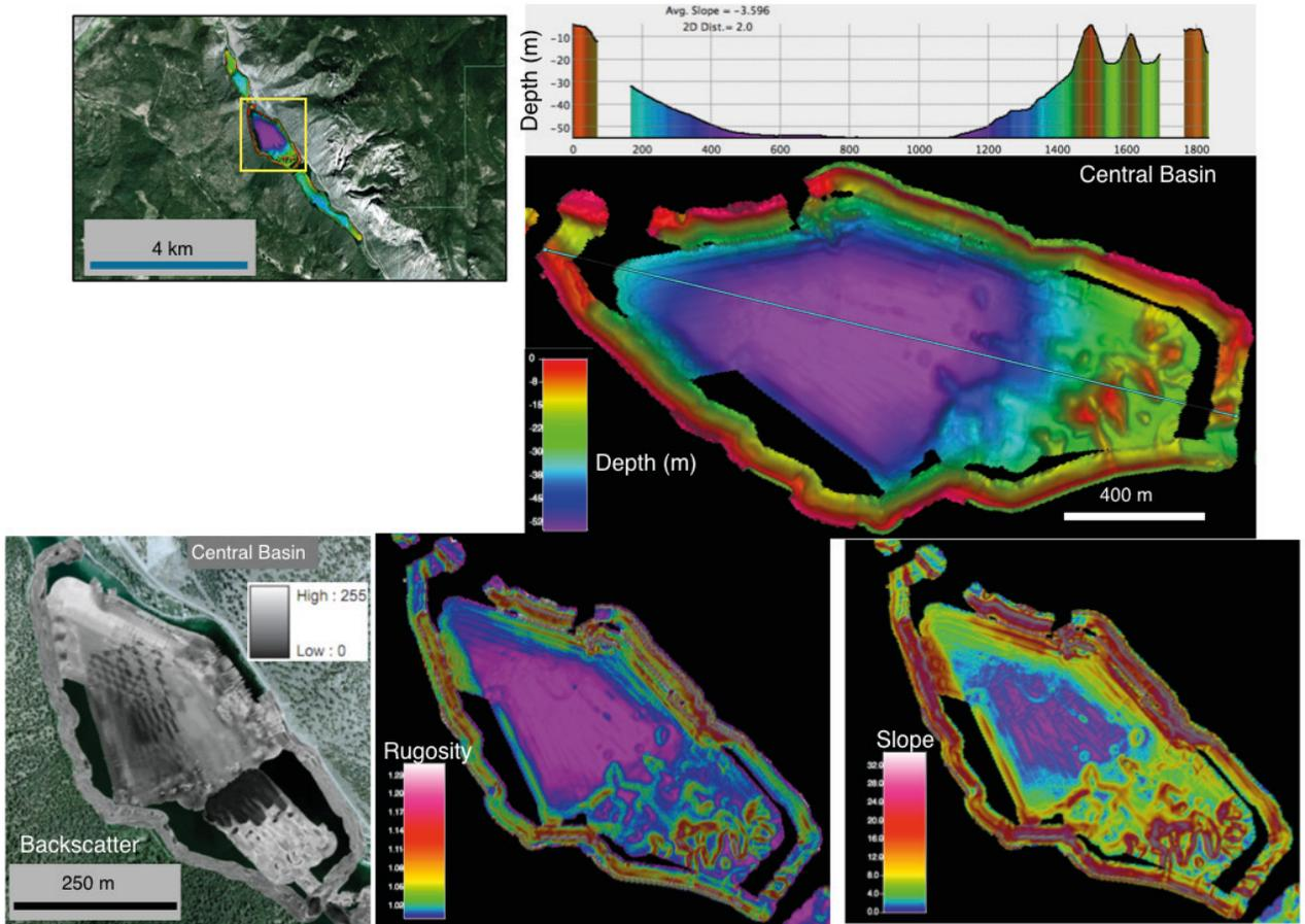
Figure 3. Geoaoustic mapping products compiled for the Central Basin including: 5 m/pixel gridded bathymetry (upper right), slope (lower right), rugosity (lower center), and 0.18 m/pixel scaled backscatter (lower left).
