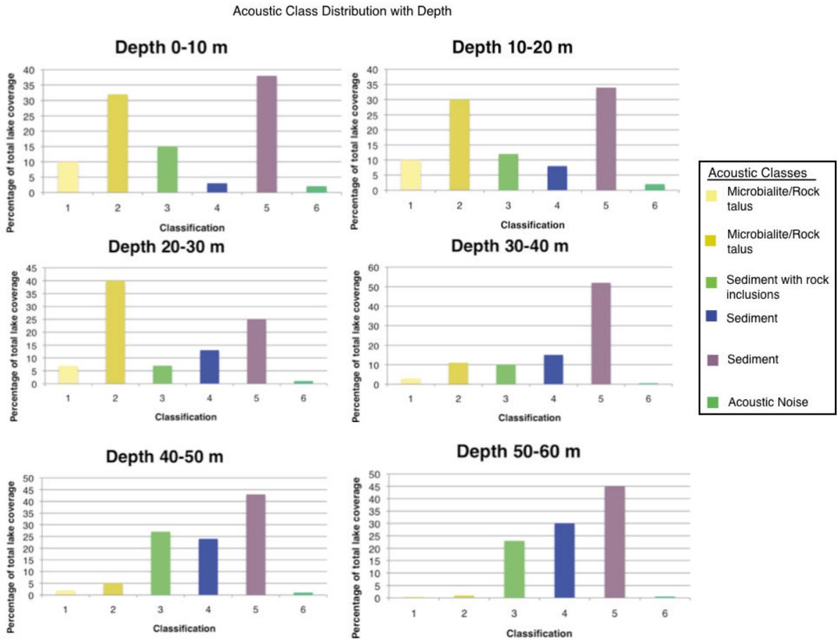
Figure 7. Distribution plots showing the percentage cover of the lake bed for each of the acoustically derived (ground truth confirmed) class types within 10 m depth intervals from the surface (upper left) to the maximum depth of the lake (lower right).
