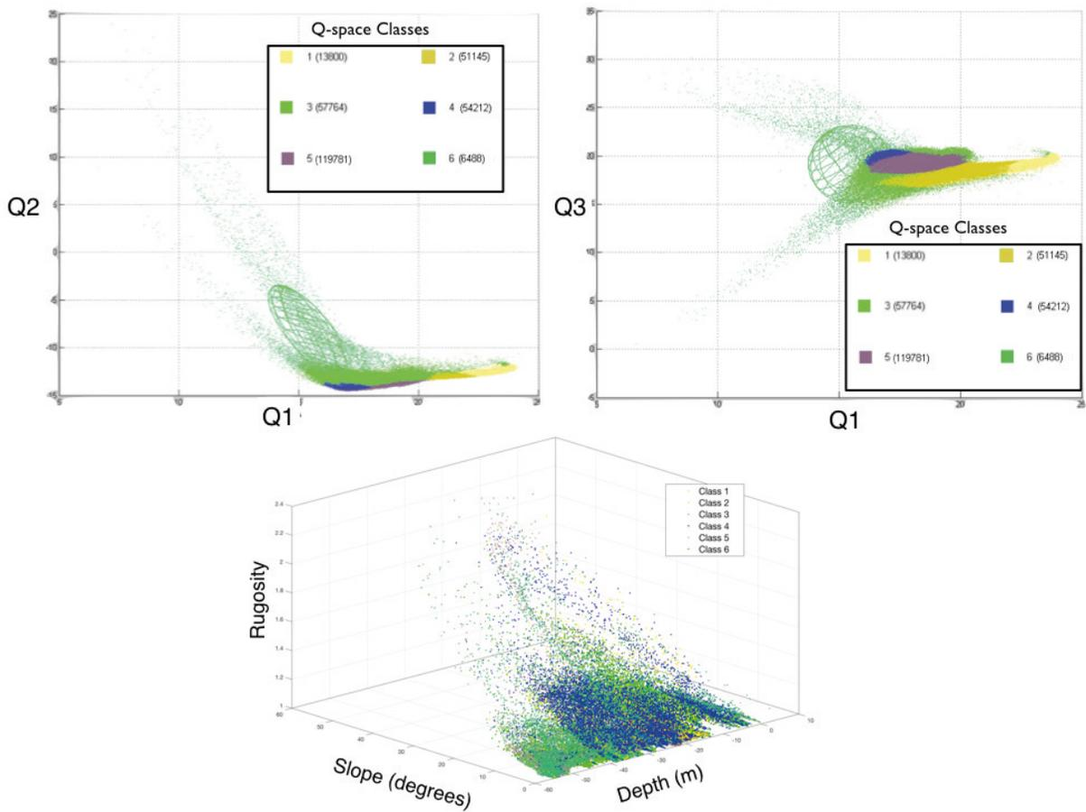
Figure 5. Principal component Q-Space view of multidimensional geacoustic data analysis displaying components Q1 and Q2 (upper left) and components Q1 and Q3 (upper right). Distribution of each of the 6 class types in relation to depth, slope, and rugosity (lower panel).
