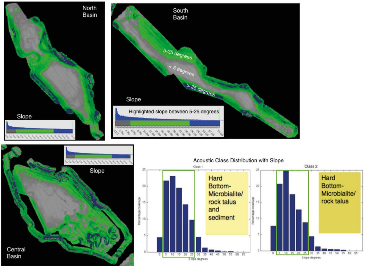
Figure 8. North Basin, Central Basin, and South Basin slope 5-25° highlighted green. The blue area is slope greater than 25°, and the gray area is slope less than 5°.
