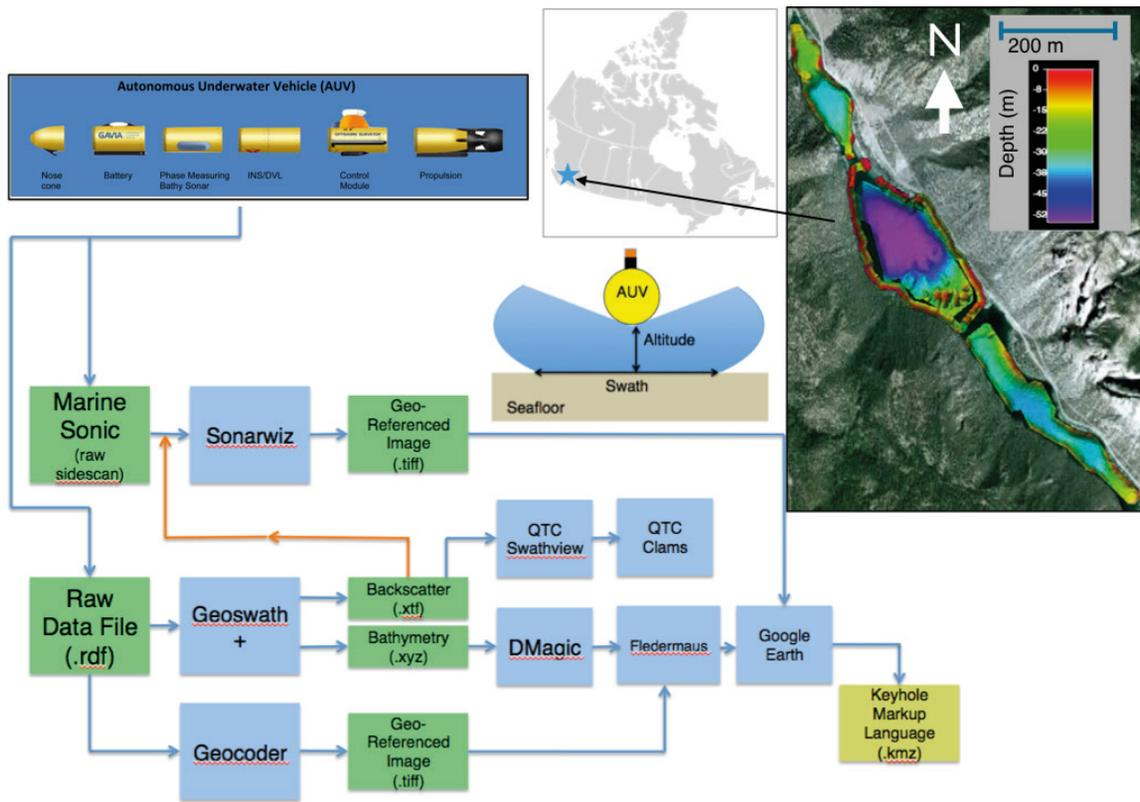
Figure 1. Site Map of Pavilion Lake (upper right) located in British Columbia Canada. Gavia AUV as configured for lake mapping (upper left) and workflow of geoaoustic data processing.
