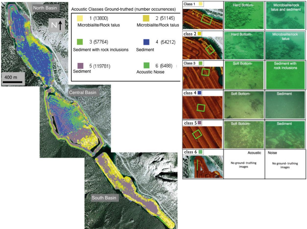
Figure 6. QTC automated backscatter classification map of Pavilion Lake (left panel). A side-scan sonar image of each classification, along with the color. Ground-truthing images collected with the DeepWorker submersible (right panel).
