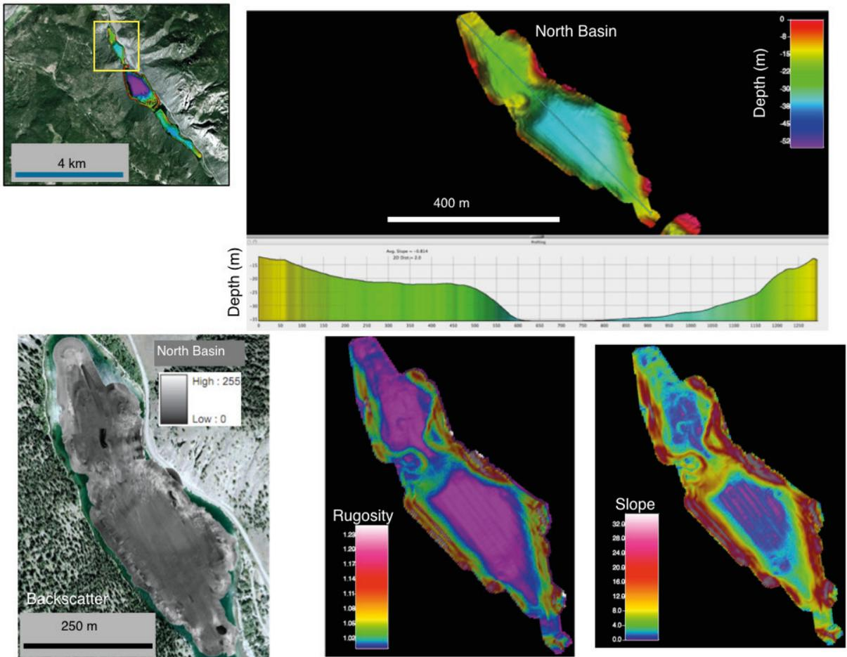
Figure 2. Geoacoustic mapping products compiled for the North Basin including: 5 m/pixel gridded bathymetry (upper right), slope (lower right), rugosity (lower center), and 0.18 m/pixel scaled backscatter (lower left).
