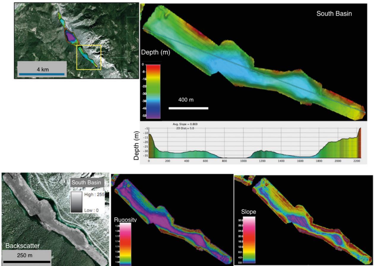
Figure 4. Geoacoustic mapping products compiled for the South Basin including: 5 m/pixel gridded bathymetry (upper right), slope (lower right), rugosity (lower center), and 0.18 m/pixel scaled backscatter (lower left).
