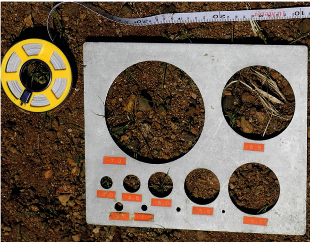
Figure 5. The template for field sieving of the coarse particles. The holes are arranged on a \frac{1}{2} phi scale.
