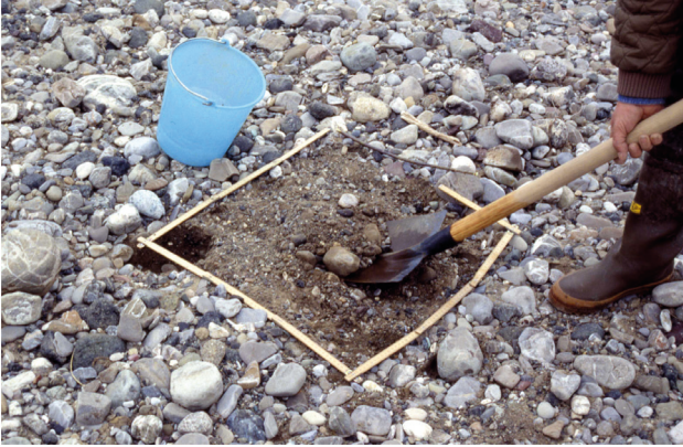
Figure 4. Collection of a subsample (black square in figure 2). Notice the armoured streambed surface and the finer sediment underneath exposed after removing the surface coarse particles.
