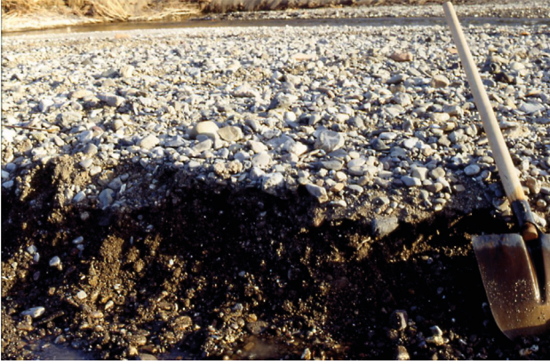
Figure 3. Example of an armoured bed. The coarse particles are concentrated on the surface, whereas the subsurface material is distinctly finer.
