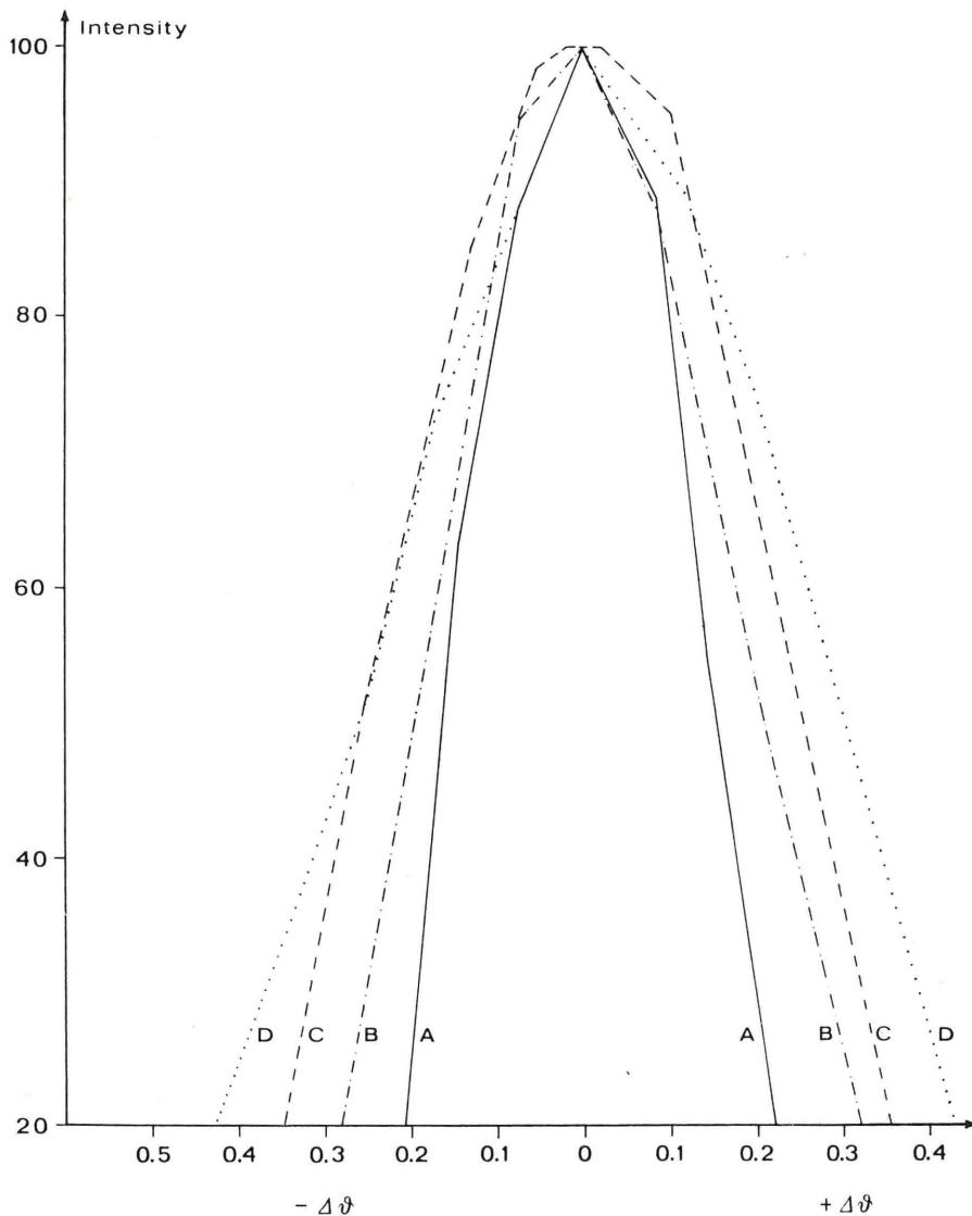
Figure 1 - Diagram showing the broadening of the  $(\bar{2}01)$  peak as a function of the dimension of the grains before homogenization. A: grains of about 0.5 cm; B: mesh grains; C: 100 mesh grains; D: very fine powder.
