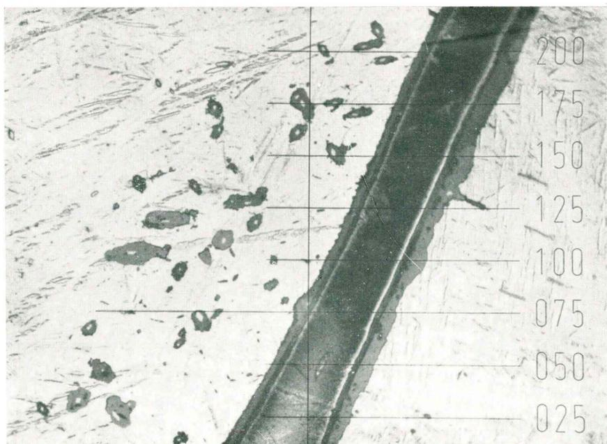
Fig. 6 - Nital 15 sec. The scale is in  $\mu$ . The dark grey band is a teanite lamella
